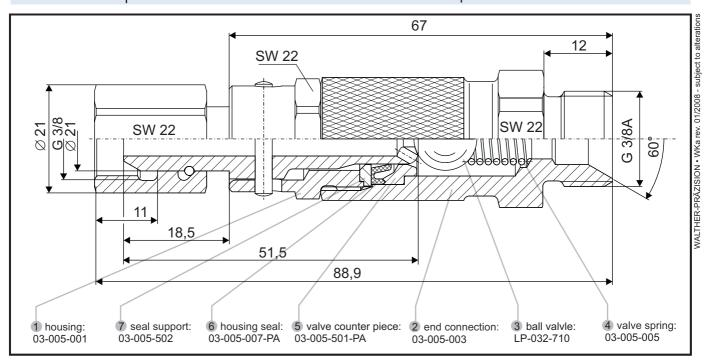
**Optional:** with other end connections, in stainless steel, as high pressure version up to max. static 200 bar working pressure
