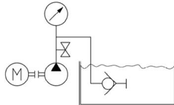
Test 3: self sealing adaptor disconnected
