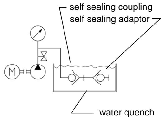
Test 2: self sealing adaptor disconnected
