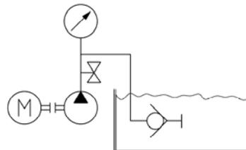
Test 3: self sealing adaptor disconnected
