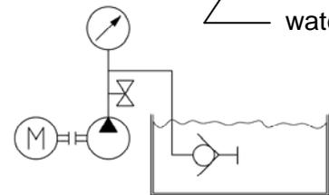
Test 3: self sealing adaptor disconnected
