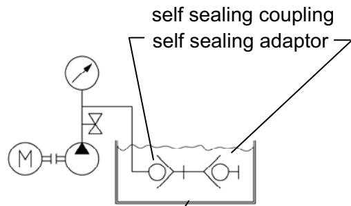
Test 2: self sealing adaptor disconnected
