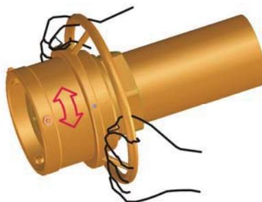
Slide the free half (adaptor) axially centred onto the plug part of the fixed half (coupling) until sensible resistance.
