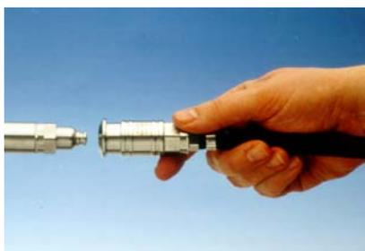
If the coupling axis does not align to the adaptor axis (inclined approach) the coupling can be centered with some feeling.
