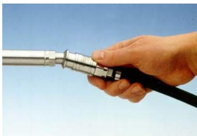
The coupling is finally slid on until mechanical end stop. In doing so the locking sleeve jumps audibly and sensibly some mm to the front (into the direction of the adaptor) and the coupling is connected and safely locked.
